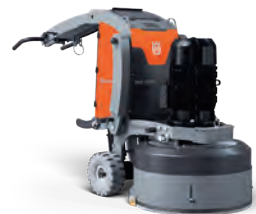
ELECTRIC-POWERED HUSQVARNA BMG 780 / BMG 780RC 15kW, 400V, 32A-63A, 3-phase, grinding width 780mm, weight 487/639kg.
