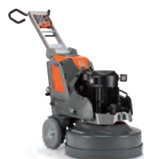
ELECTRIC-POWERED HUSQVARNA PG 830 RC 16.5kW, 380-415V, 3-phase, grinding width 800mm, grinding disc 3 x 270mm, 598kg.
