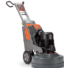
ELECTRIC-POWERED HUSQVARNA PG 830 16.5kW, 380-415V, 3-phase, grinding width 800mm, grinding disc 3 x 270mm, 556kg.
