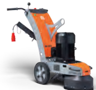
ELECTRIC-POWERED HUSQVARNA BG 250 5.5kW, 400V, 3-phase, grinding width 250mm, 146kg.
