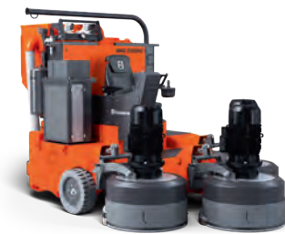
ELECTRIC-POWERED HUSQVARNA BMG 2200 63kW, 400V, 125A, grinding width 2200mm, grinding disc 3x3, 3035kg.
