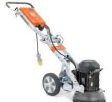
ELECTRIC-POWERED HUSQVARNA PG 280 3-2.2kW, 400-220V, 3-phase/1-phase, grinding width 280mm, 70kg.
