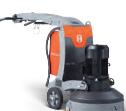
ELECTRIC-POWERED HUSQVARNA BMG 555 7.5kW, 400V, 16A, grinding width 555mm, 298kg.
