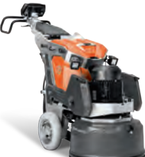
ELECTRIC-POWERED HUSQVARNA HTC X6 / HTC RX6 7.5kW, 380-415V, 3-phase, grinding width 600mm, grinding disc 3 x 230/4 x 230mm, 384/441kg.
