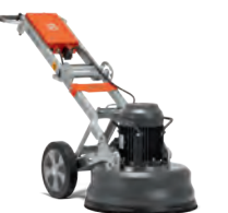
ELECTRIC-POWERED HUSQVARNA PG 510 4.0-2.2kW, 400-220V, 3-phase/1-phase, grinding width 515mm, grinding disc 3 x 230mm, 133/120kg.
