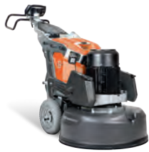
ELECTRIC-POWERED HUSQVARNA HTC X8 / HTC RX8 12-15kW, 380-415V, 3-phase, grinding width 800mm, grinding disc 3 x 270/4 x 270mm, 499/574kg.
