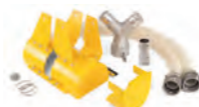
DUST SUCTION COVER KIT A cover and hose kit for the ER 50 drum cutter to enhance the work environment by reducing airborne dust and smaller particles. The dust suction cover is placed around the cutting heads. Can be retro-fitted to the ER 50 drum cutter.
