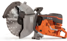
PETROL-POWERED HUSQVARNA K1270 SMARTGUARD 119cc, 5.8kW, 15.1kg, blade size 400mm, cutting depth 118/145mm.
