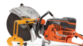
PETROL-POWERED HUSQVARNA K1270 RAIL 119cc, 5.8kW, 20.5/21.2kg (incl. RA10), blade size 350/400mm, cutting depth 118/145mm.
