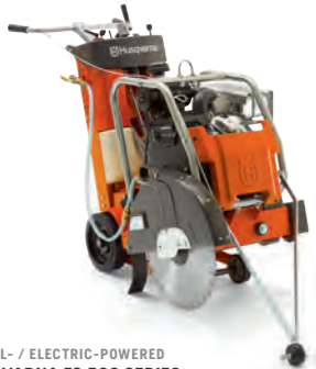
PETROL- / ELECTRIC-POWERED HUSQVARNA FS 500 SERIES Diamond blade max 600/500 mm, cutting depth 241/179 mm, 231/197. FS 524, petrol, 15.5 kW*. FS 513, petrol, 8.7 kW*.
