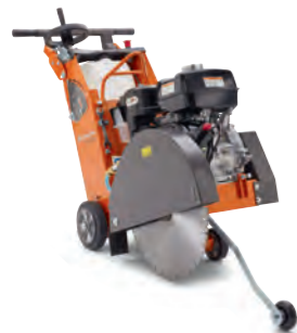
PETROL-POWERED HUSQVARNA FS 400 LV Diamond blade max 450/500 mm, cutting depth 162/189 mm, 99/120 kg, 8.7 kW*.
