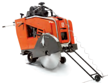
ELECTROHYDRAULIC-POWERED HUSQVARNA FS 4800 D Diamond blade max 900 mm, 680–695 kg, cutting depth 381 mm, 35 kW*.
