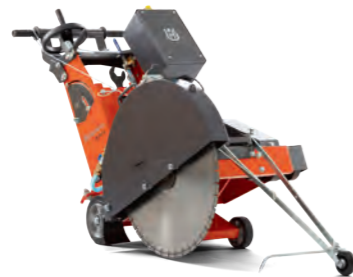
ELECTRIC-POWERED HUSQVARNA FS 600 E / FS 500 E Diamond blade max 600/500 mm, cutting depth 240/192 mm, 178/145 kg, 7.5 kW*.
