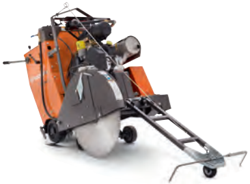
ELECTROHYDRAULIC-POWERED HUSQVARNA FS 3500 EFI G Diamond blade max 750 mm, 419 kg, cutting depth 311 mm, 27.5 kW*.
