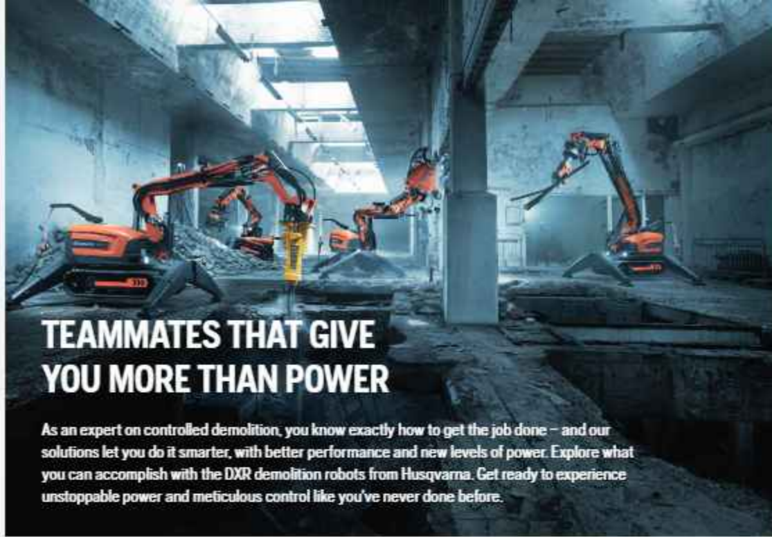
HYDRAULIC-POWERED HUSQVARNA DXR 95 9.8 kW, 589 kg, reach 3.2/2.7 m up/forward incl. tool.
