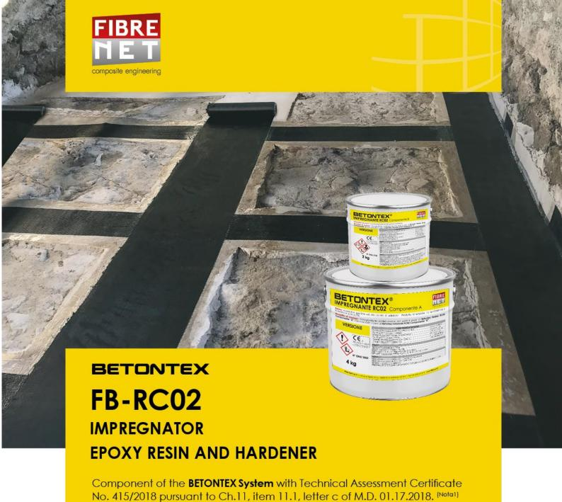
**FB-RC02** Thixotropic epoxy resin with adhesive and impregnating function for the application of tapes, fabrics or nets to the substrate to be reinforced. The product is supplied in two components, the resin and the hardener, whose dosage must be made by weighing in a 2:1 proportion.
