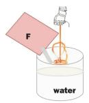
For mixing of single bags, it is acceptable to use a 25 litre steel pail as a mixing vessel, and mixing carried out using a slow speed electric drill (350/360 rpm) fitted with
