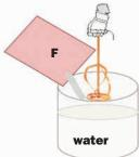
For mixing a single bag, a 25 litre steel pail is suitable, using a slow speed electric drill (350/600rpm) fitted with a **SpECbuild Mixing Paddle**. Where larger
