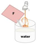
For mixing a single bag, a 25 litre steel pail is suitable, using a slow speed electric drill (350/600rpm) fitted with a **SpECbuild** Mixing Paddle. Where larger
