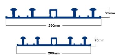
**External Construction Joint (ECJ)** sections are used in construction joints and incorporate grout excluding fins to give a positive area to locate formwork and control grout loss.
