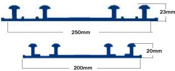
**EEJ** and **ECJ** sections incorporate a nailing flange with a reinforced edge to provide secure fixing that will resist tearing.
